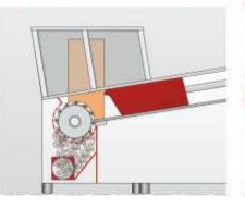
Rotor with diameter 354 mm for higher throughput
