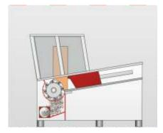
Rotor with diameter 252 mm for smaller applications
